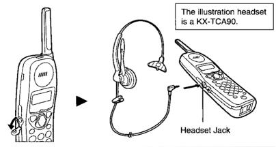
When an optional headset is connected to the handset, make sure to use the headset to talk with the caller. If you want to have a normal cordless phone conversation, disconnect the headset.
