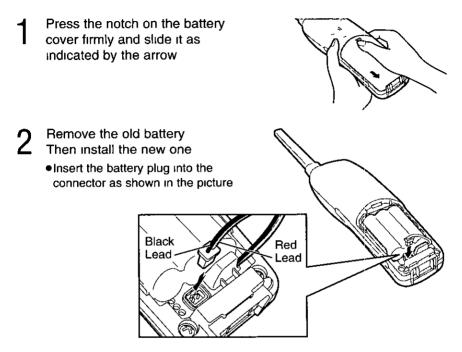
3 Close the cover Make sure you charge the new battery for about 15 hours in order to display the battery strength prompt correctly (p 14)
